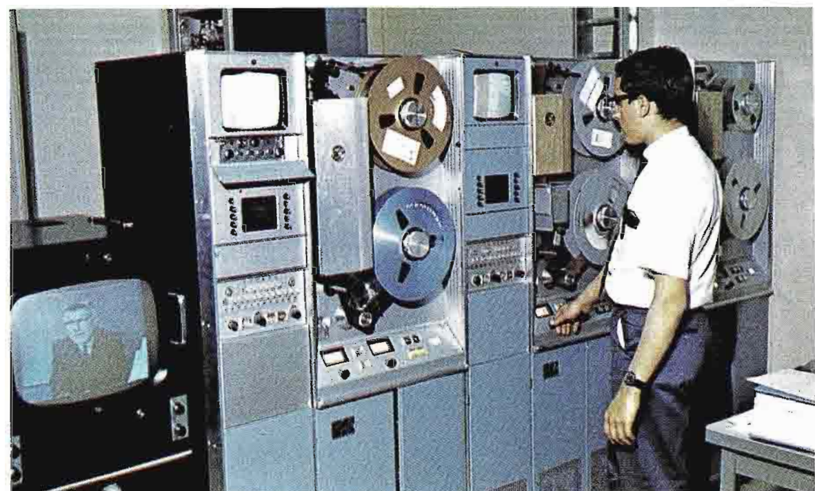
FIG. 8 Studio engineer checks the playback of program on the TR-50 highband color recorder. To the right are the two TR-4 recorders. Not shown is the TR-5 mobile recorder used both in the studio and their mobile van.
