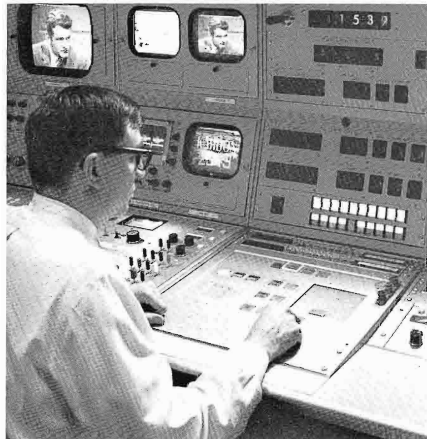
FIG. 11 Automation remote console—showing read-in panel, where program log information is recorded in memory for upcoming station breaks.
