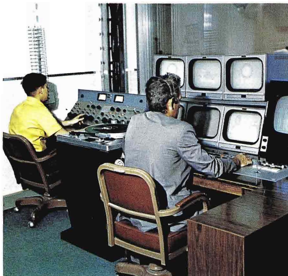
FIG. 12 Compact arrangement of studio controls showing audio operator at the BC-7 console, and video operator at the TS-40 switcher.
