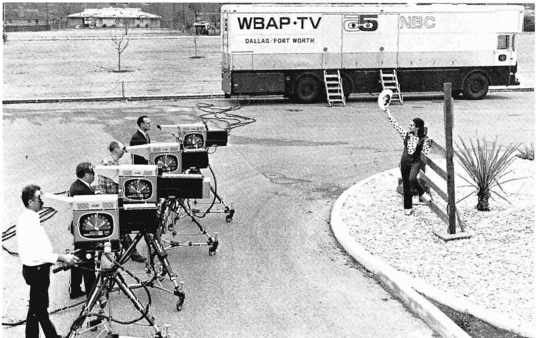
FIG. 1 The first four TK-44A cameras shown here are being used in WBAP-TV's big mobile TV unit for covering remotes. Additional TK-44A's have been added for studio programs.
